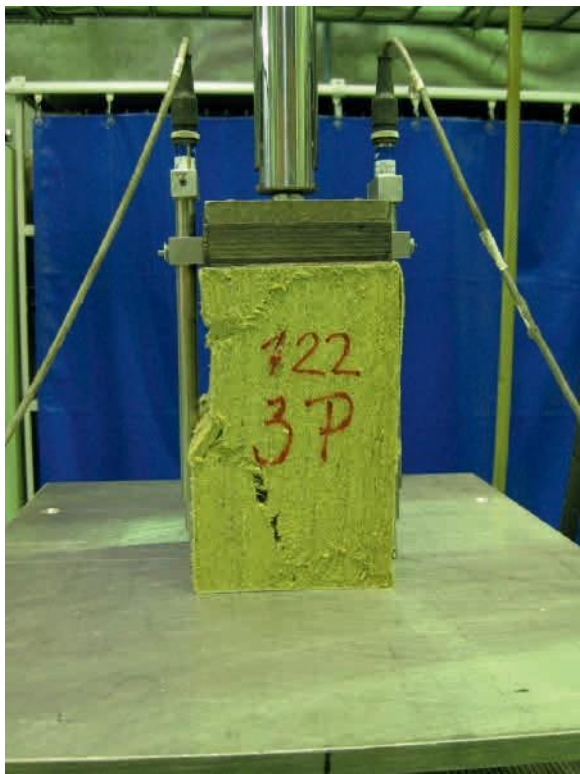
Figure 12: Compression test failed specimen
