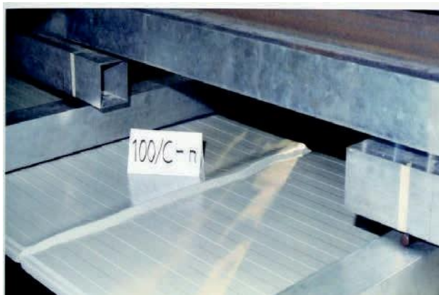
Figure 20: Wrinkling of a lightly profiled face (negative orientation)
