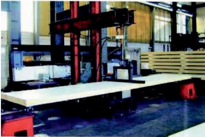
Figure 24: Internal support bending test with regular loading
