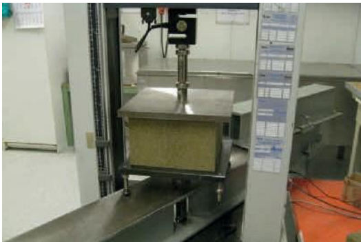
Figure 11: Test of compressive strength and compressive modulus
