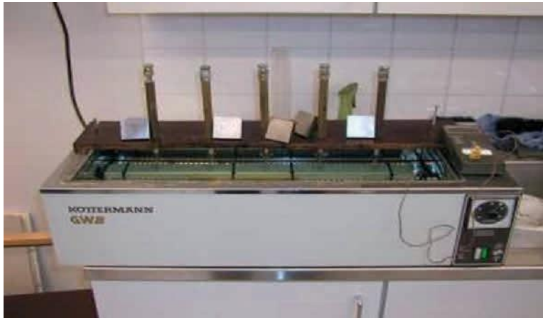
Figure 36: Wedge test arrangement
