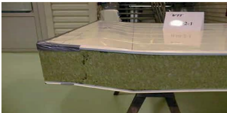
Figure 35: Failure of a specimen in a support reaction test (the final failure was shear)
