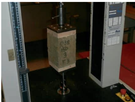
Figure 13: Cross-panel tensile test - measurement of the movement from loading bridge
