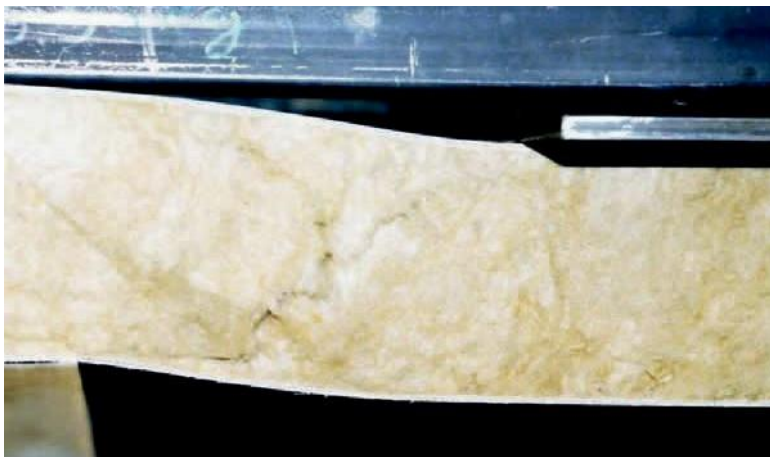
Figure 7: Shear tests on short beams of MW cored panels
