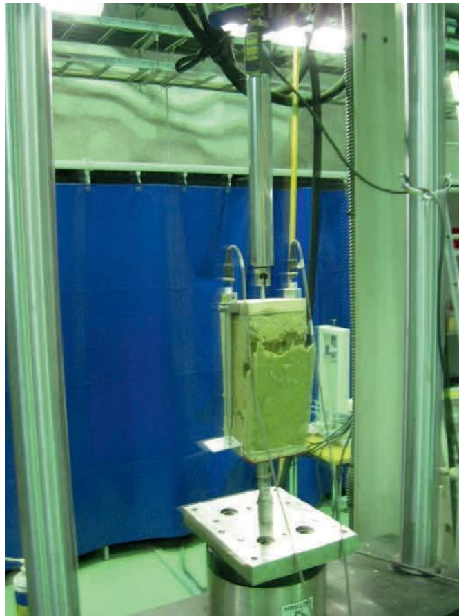
Figure 14: Cross-panel tensile test - measurement of the movement directly from specimen
