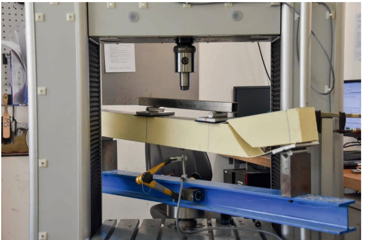
Figure 6: Shear tests on short beams of PU cored panels
