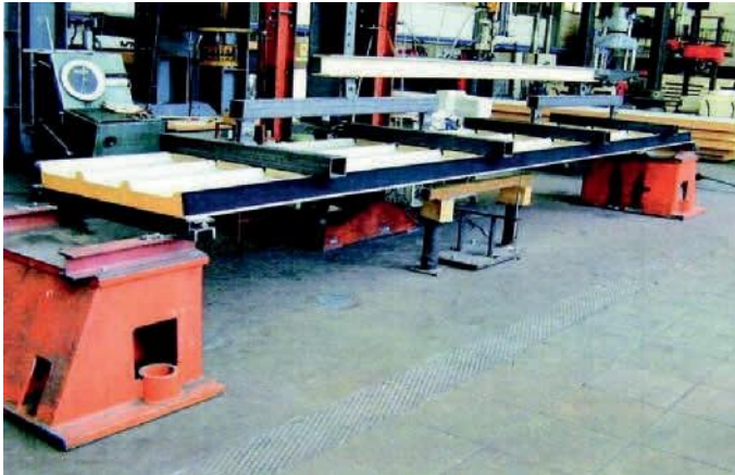
Figure 17: Bending test arrangements based on line loads. Loads shall be introduced on the lower parts of the face profile.
