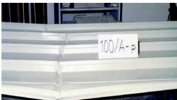
Figure 21: Buckling of the trapezoidal face (positive orientation)
