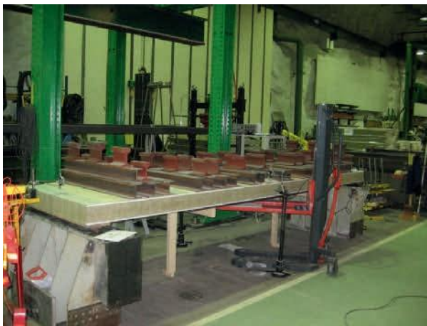
Figure 26: Creep coefficient test set-up
