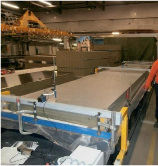
Figure 19: Test set-up in partial vacuum bending test
